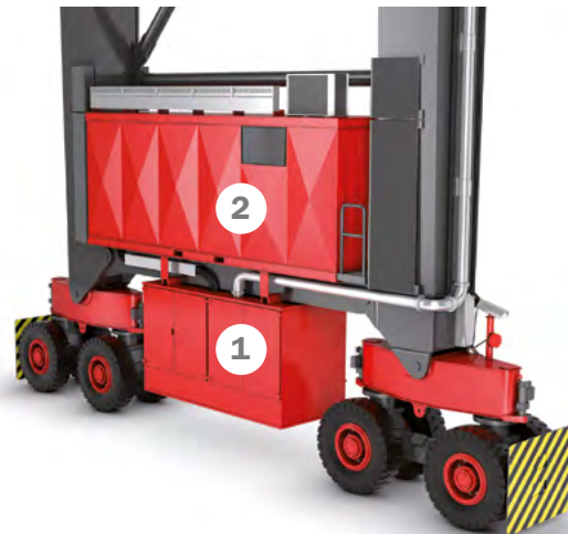
Figure 2. The diesel fuel saver is retrofitted in the genset enclosure (1) while the necessary modifications to the electrical systems are made in the e-house (2) above it. Some software modifications are also done at the same time.
